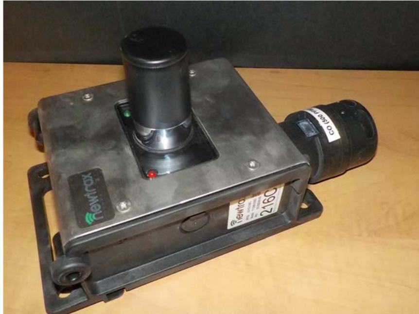
Figure 2: A Newtrax-Enabled Conspec Smart Head Wireless Carbon Monoxide (CO) Gas Transmitter. 2a – Remote Monitoring using Wireless Carbon Monoxide Gas Transmitters
